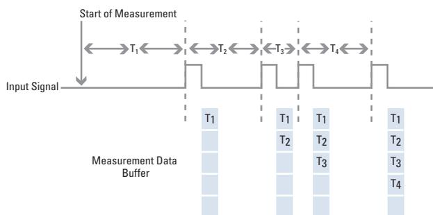
Figure 1. Buffered Period Measurement with Counter/Timers
