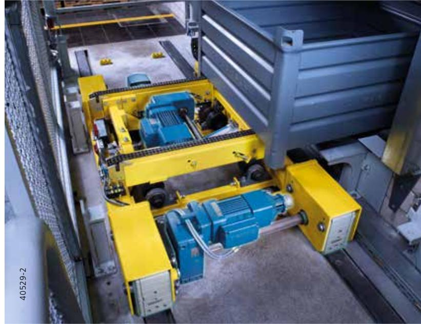
Furthermore, the patented torque bracket enables torque to be transmitted from the geared motor to the wheel block without any radial force. This reduces the load on the drive shaft and extends its service life.
