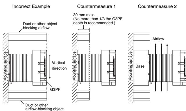
If the depth direction of the G3PF is obstructed by ducts, the heat radiation will be adversely affected.
