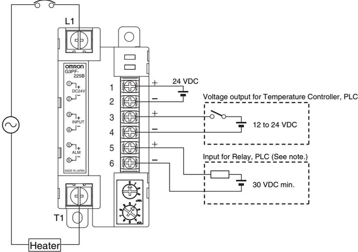
Note: With inductive loads (relay coil, etc.), connect back-current prevention diodes to both sides of the load.
