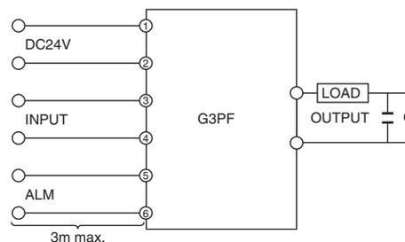
Recommended capacitor: 1 μF, 250 VAC for the G3PF-2□□B, and 0.5 μF, 500 VAC for the G3PF-5□□B
