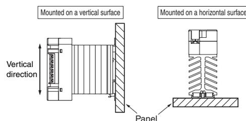
7. When mounting the G3PF to a control panel or other fixture with screws, be sure to tighten the screws to a torque of 0.98 to 1.47 N·m. A lower level of tightening torque may cause the G3PF to fall.
