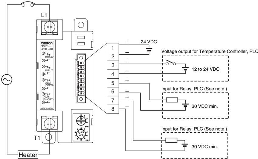
Note: With inductive loads (relay coil, etc.), connect back-current prevention diodes to both sides of the load. Terminals 5-6 output a heater burnout alarm, and terminals 7-8 output an SSR short-circuit failure alarm.
