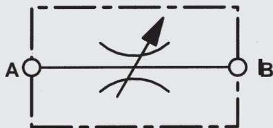
Flow control valves with reverse flow check DRV
