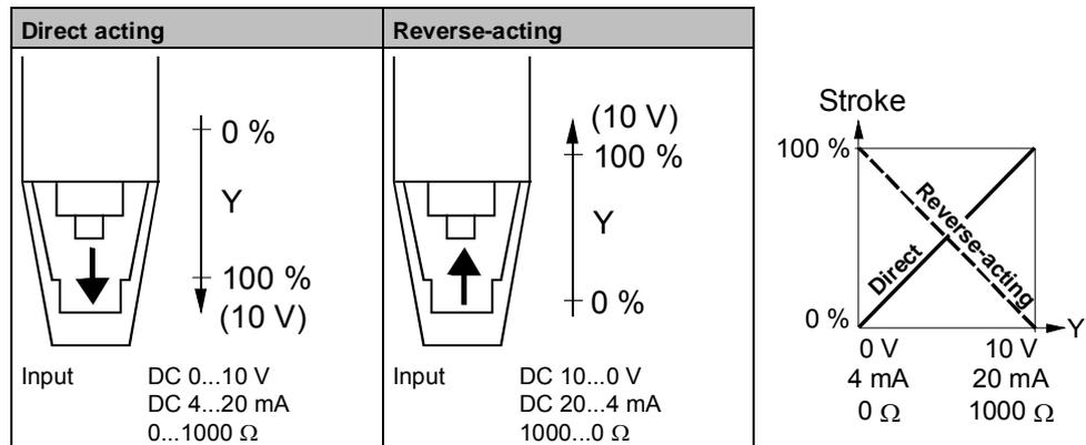
Note The mechanical spring-return function is not affected by the direction of operation selected.
