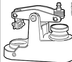
0 % actuator stroke corresponds to 100 % valve stroke; mount between valve and actuator
