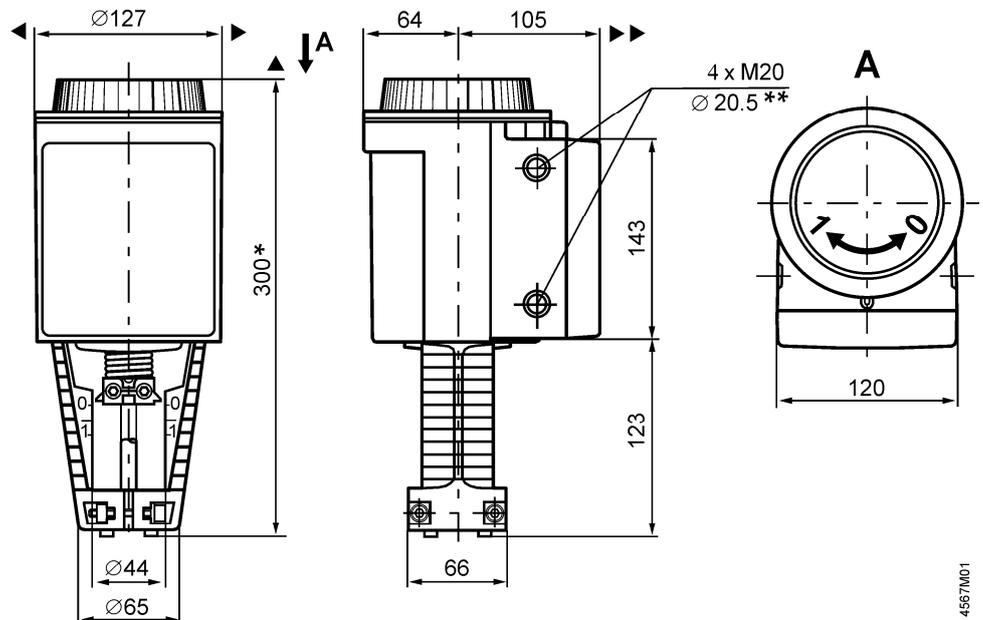
\* Height of actuator from valve plate without stroke inverter **ASK50 = 300 mm**
