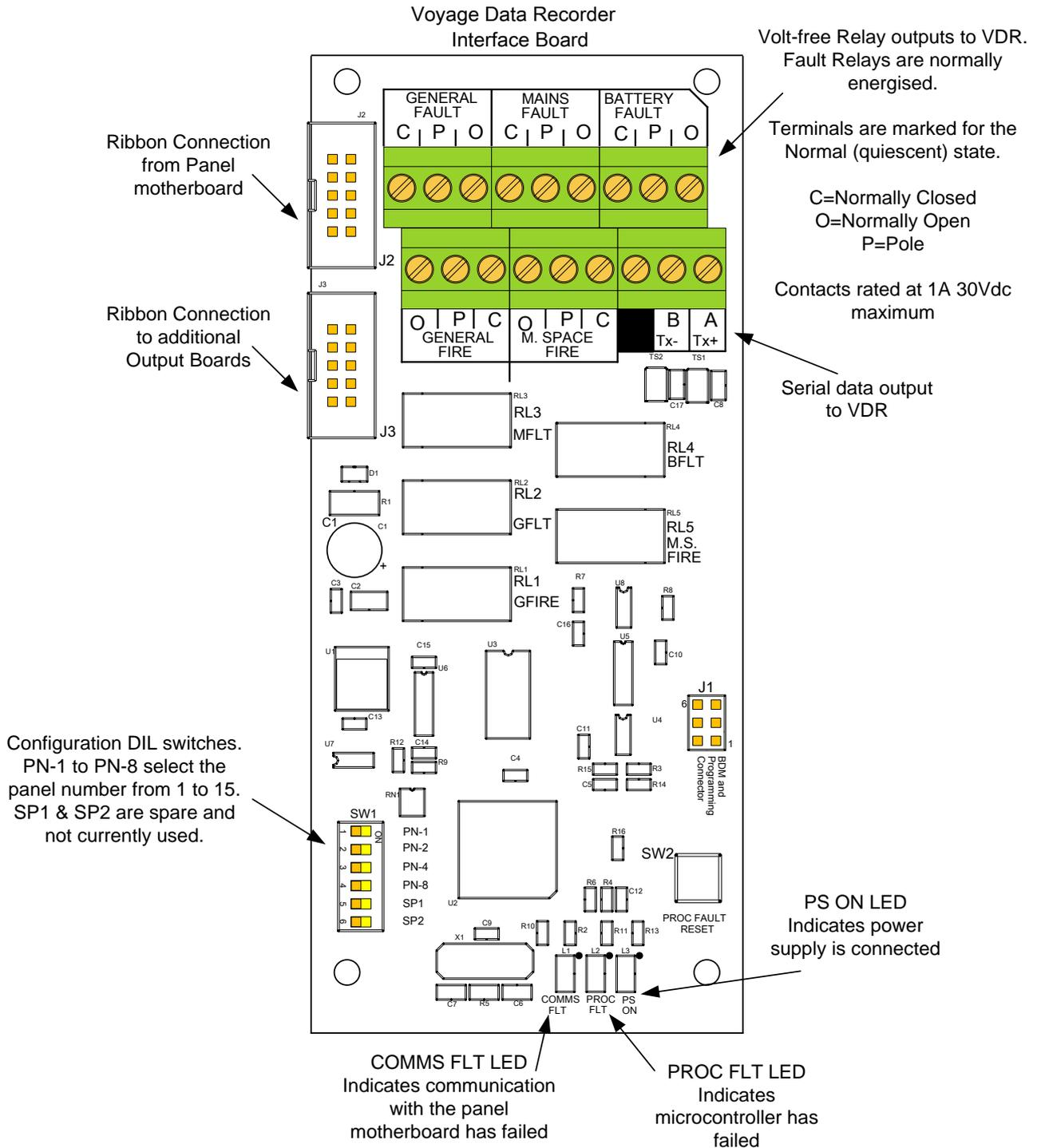
**Figure 12 – C1714 VDR Output Module PCB Layout**
