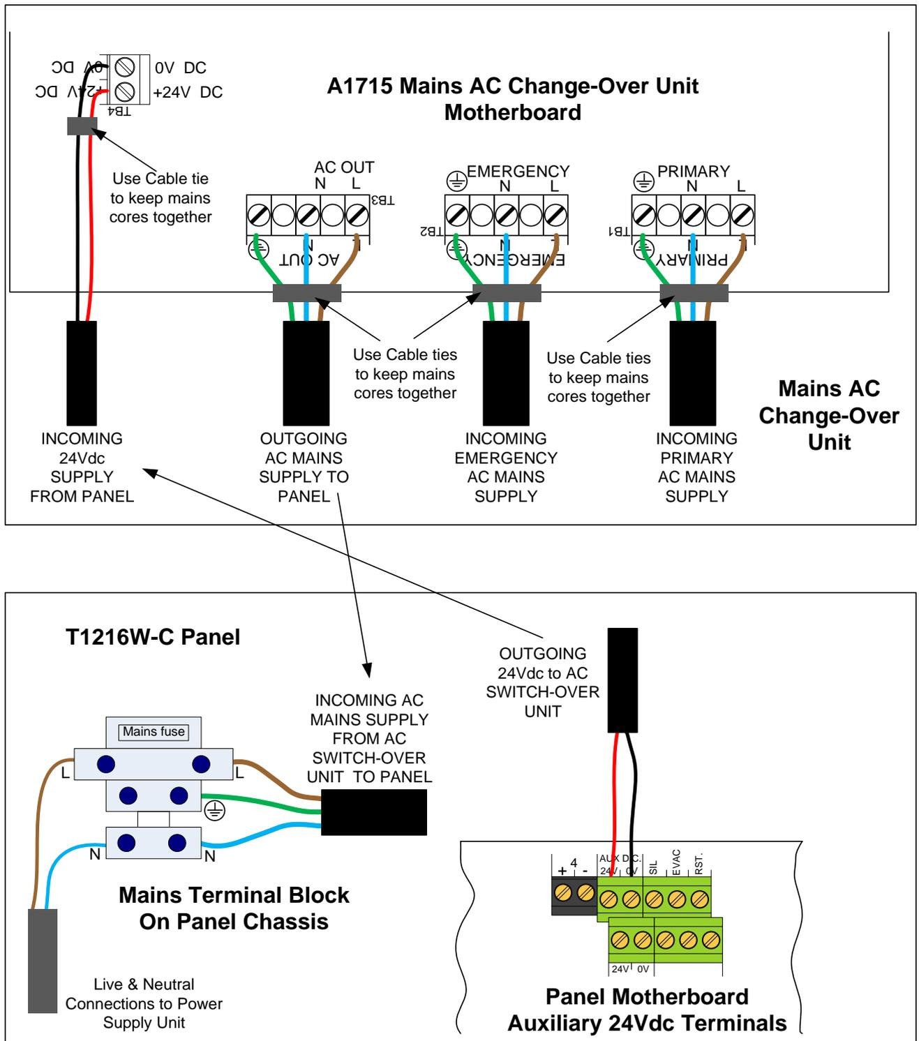
**Figure 20 – Mains AC Change-Over Unit Electrical Installation Diagram**
