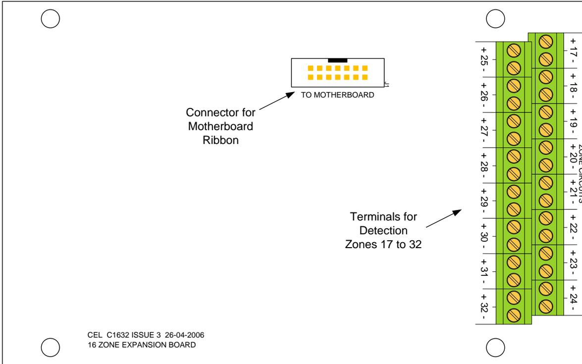
**Figure 10 – C1632 16 Zone Expansion Board Layout**
