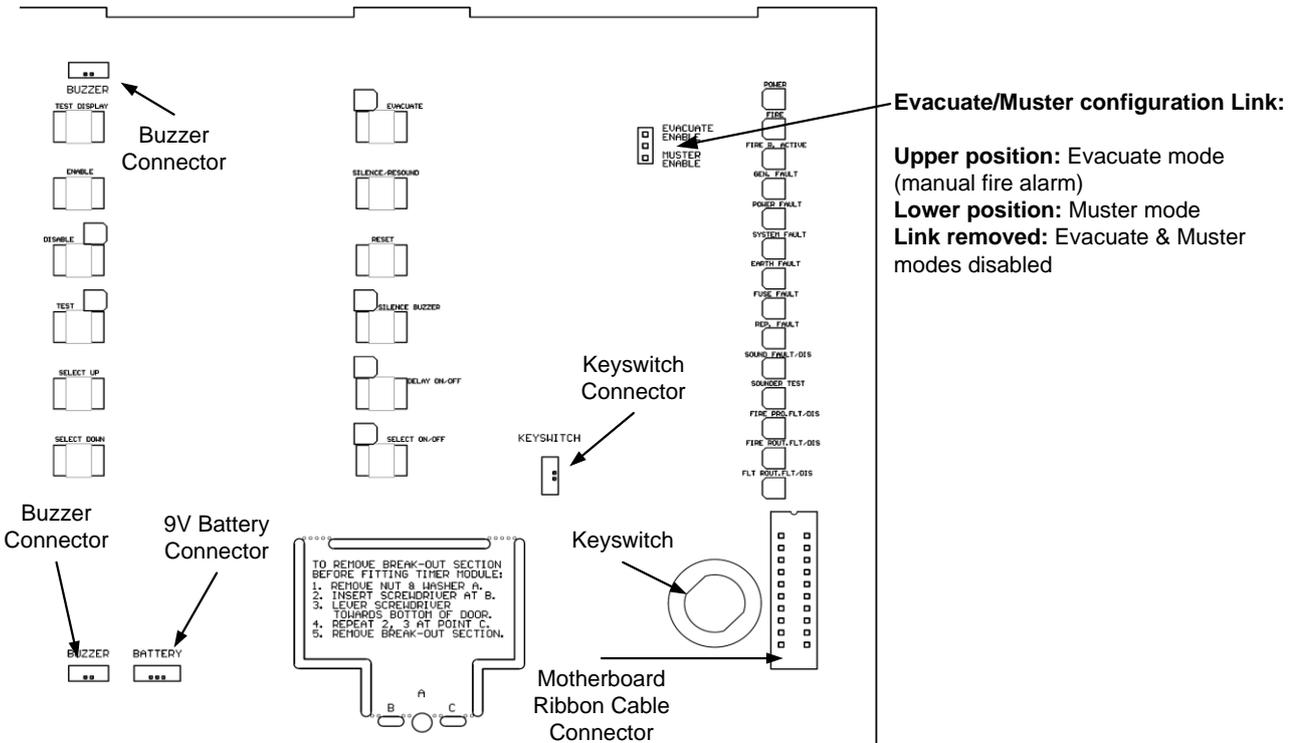
**Figure 11 – Rear Right Hand Side of Display PCB**
