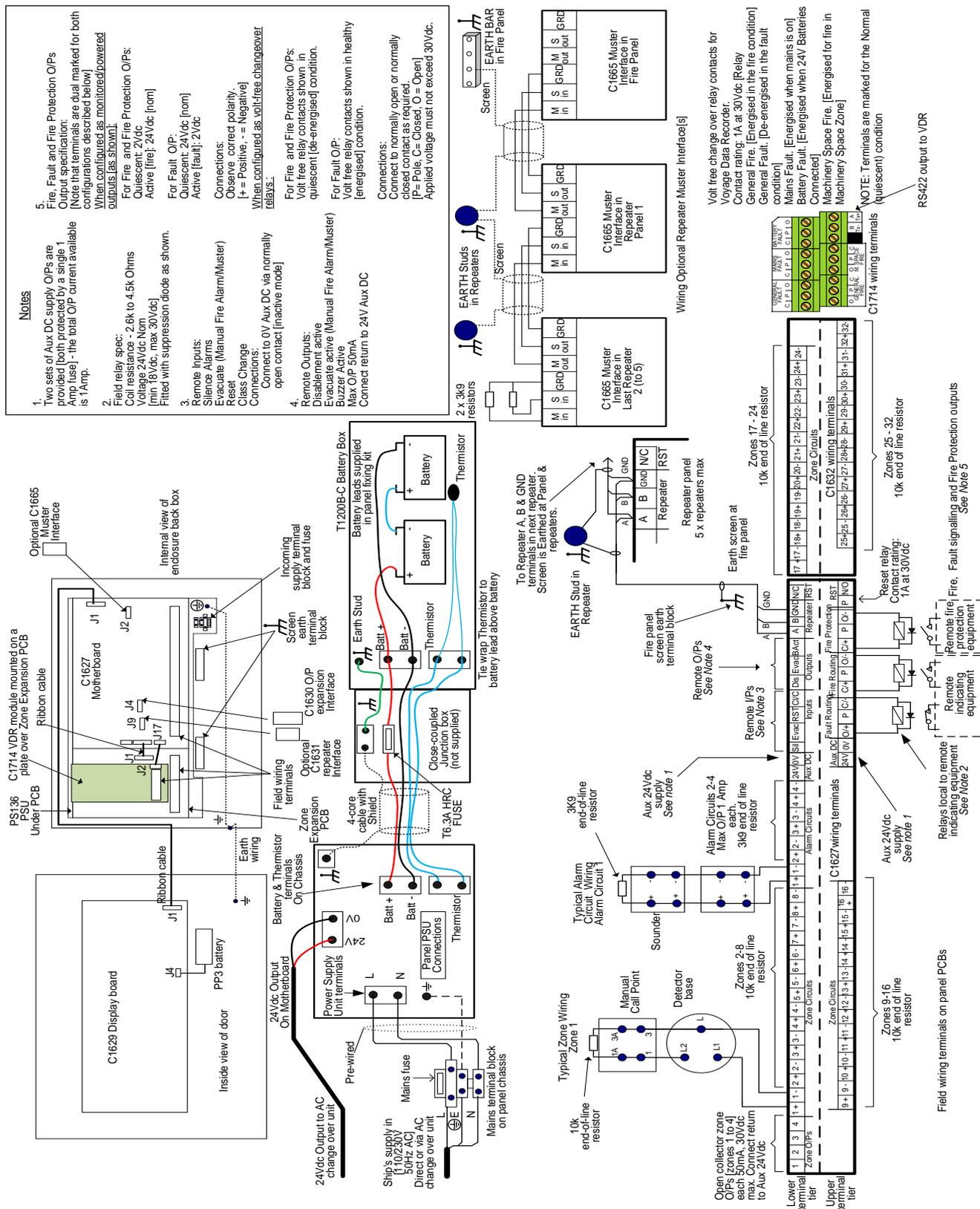
Figure 22 – T1232-C Electrical Installation Diagram
