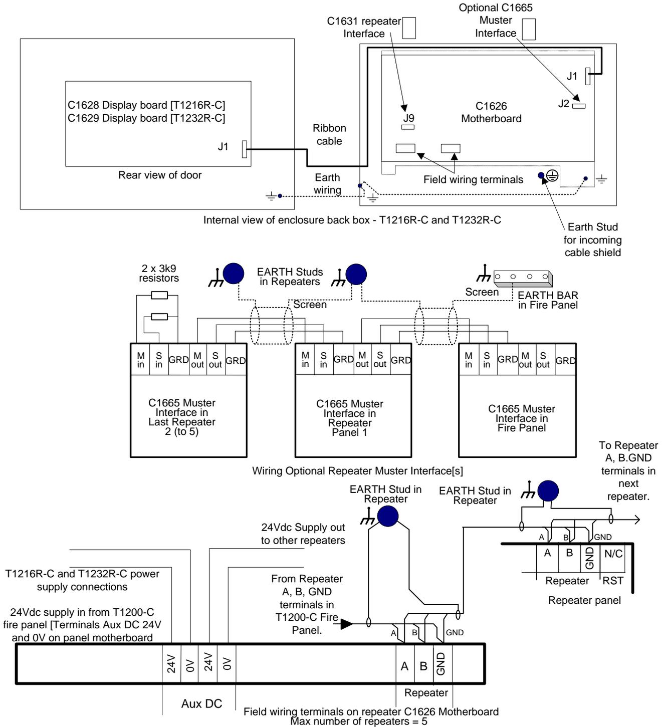
Figure 25 – T1216R-C/T1232R-C Repeater Electrical Installation Diagram
