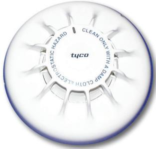
The MR601TEX overcomes the slower response of optical detectors to hot burning fires by increasing the sensitivity of the optical detector when it is associated with a rapid change in temperature. In this way it is intended to become a detector which will suit some of the risks currently covered by ion chamber detectors. Smoke detectors will not detect burning alcohol or other clean burning liquids which do not generate smoke particles.
