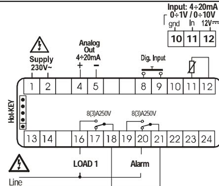
Probe: Pt100=11 - 10 (12); Thermocouple J, K, S = 11(+)- 10(-)
