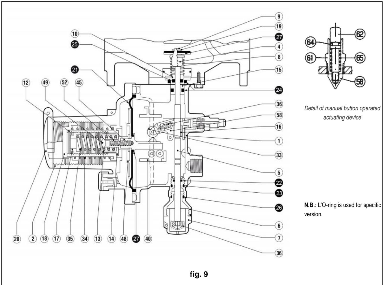
The slam-shut valve **LAV** consists essentially of an obturator (fig. 9) fitted on a stem, a releasing lever system, a control head and a manual resetting system. The pressure to control Pd, in chamber C of the control head, acts on the diaphragm 46 which is integral with the cam shaft 45.
