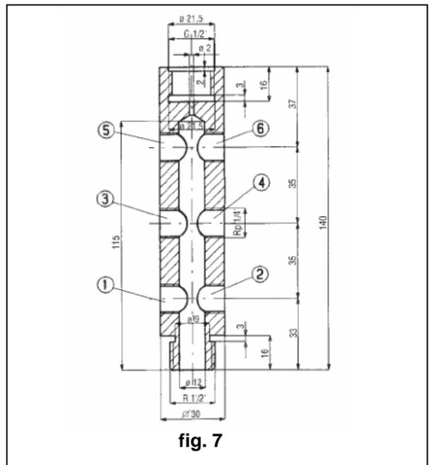
The installation of a multiple plug on a plant has its aim in in taking from a single point all the pressure impulse signals that go to the different reduction- safety devices and to their accessories.
